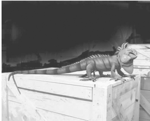
FIGURE 1.5 Iguana, an animatronics entertainment robot. (Courtesy of Stephen C. Jacobsen, SARCOS. With permission.) An animatronics character in the form of an iguana, operates on a daily basis at the RC Willey Restaurant.
